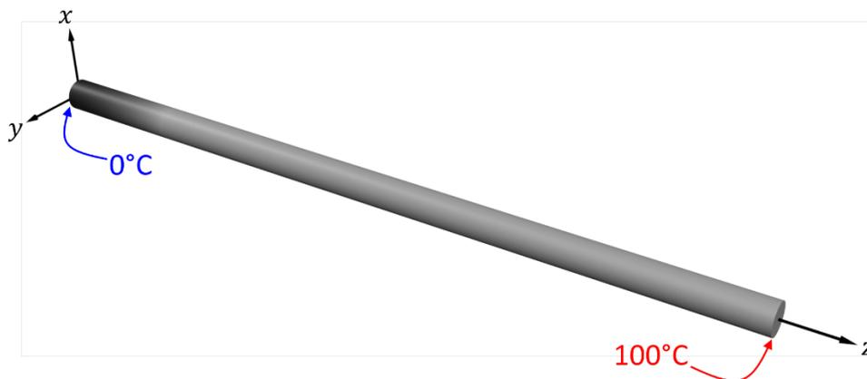
To help reconcile the physics of this problem, a function `simbartemp()` was written in MATLAB to simulate the thermal behavior of the bar and calculate the temperature  $T$  at any position  $z$  in the range  $0 \text{ m} \leq z \leq 0.6 \text{ m}$ . Calculation time is roughly 30 seconds for every value of  $z$  that must be calculated.
