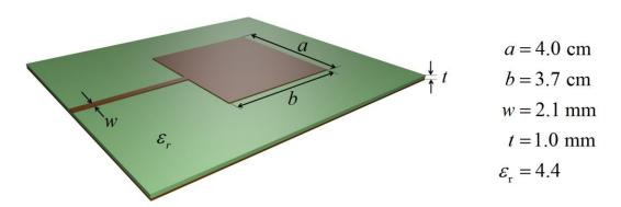
Design a quarter-wave impedance matching network for this circuit. Use tlcalc() to analyze and design the transmission line for the matching network. Be sure your design is as simple and easily manufactured as possible. Provide the following items:
