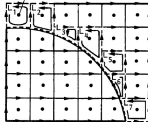
Fig. 3. Cell deformation in vicinity of a curved boundary.
