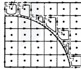
Fig. 3. Cell deformation in vicinity of a curved boundary.
