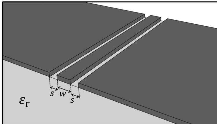
During Homework 10a and 10b, you will develop a program to analyze this transmission line using a two-dimensional finite-difference method and calculate the transmission line parameters including the distributed capacitance  $C$ , distributed inductance  $L$  and characteristic impedance  $Z_0$ .
